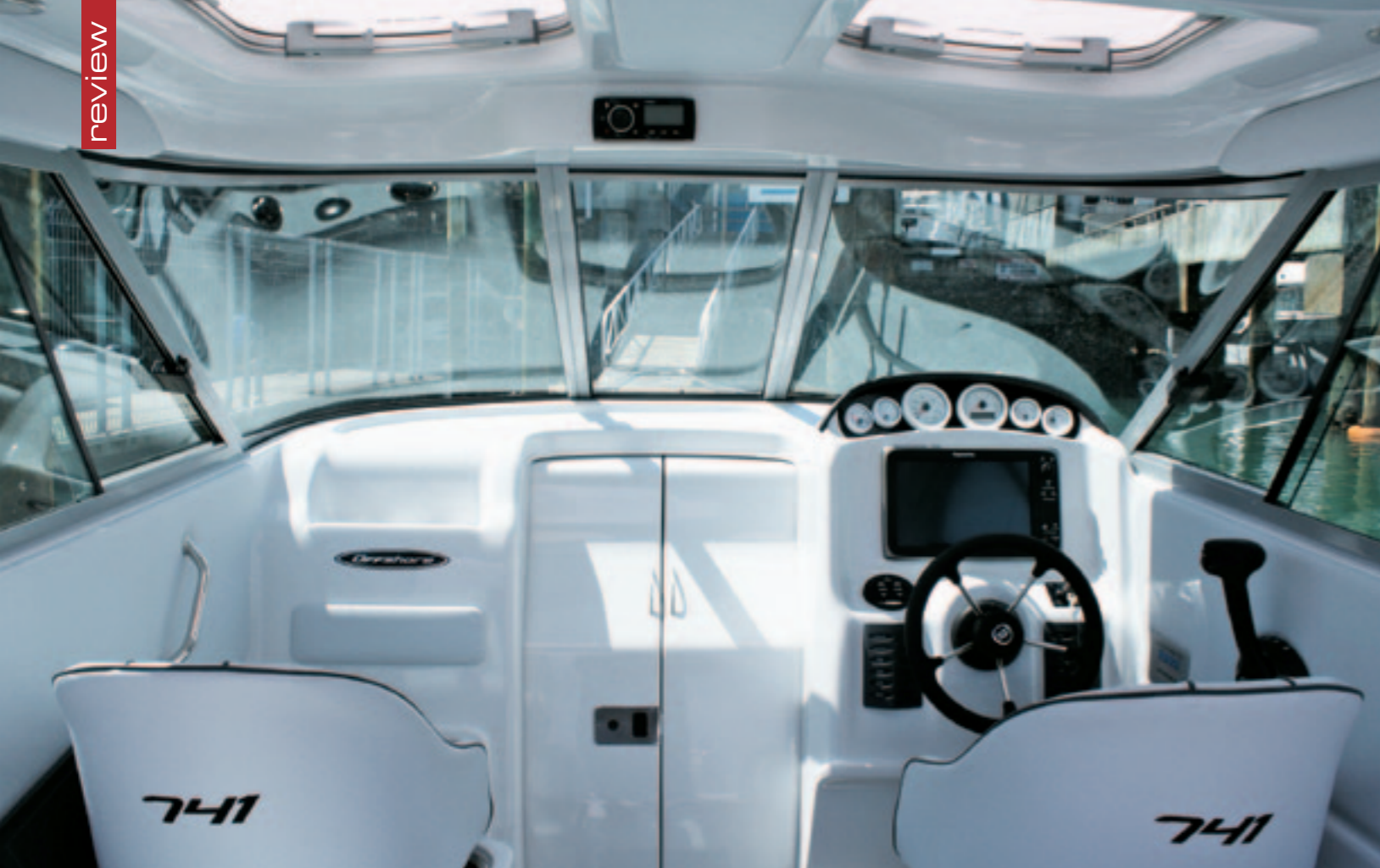
TOP: ROOF HATCHES PROVIDE EXTRA LIGHT INTO THE HELM AREA.
